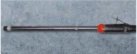
Length:approx. 615 mm10Diameter:47 mmWeight:approx. 2,1 kgDrive:vane motor
