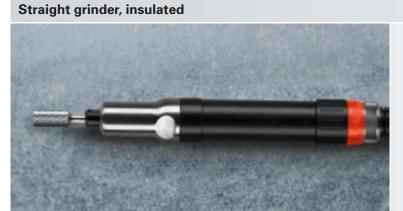
Length: approx. 206 mm **Body diameter:** approx. 30 mm Spindle casing diameter: approx. 23 mm Weight: approx. 0,40 Kg Drive: vane motor Partial front exhaust (can be restricted)
