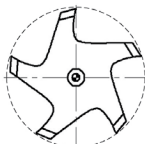
5-Punkt-Messung 5-point measuring
