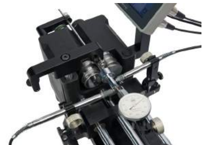
Anwendung Induktivtaster Example of use inductive probe
