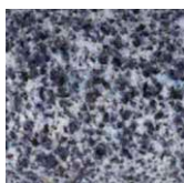
NDW Mixture of regular aluminium oxide, dark red aluminium oxide and white monocrystal aluminium oxide
