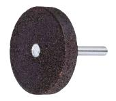
Cast materials are generally rough machined. The skin contains inclusions of sand from the casting process; large burrs, sprues and risers, holes and cracks must all be removed by grinding. Mounted points for machining cast materials must therefore be correspondingly well matched and adapted to the material. The NK hard mounted point for grinding cast materials contains special grain combinations and a tough bonding, delivering excellent performance in the applications mentioned above.
