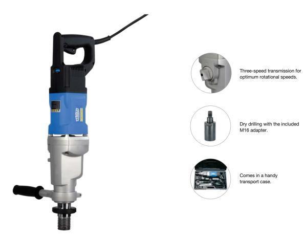
The DME22SU<sup>\*\*</sup> drill motor is ideal for electrical and installation work. It features a 3-speed transmission and variable speed setting with soft start. Integrated overload cut-outs and the PRCD safety switch ensure safe working. Dry drilling is also possible with the included M16 adapter.
