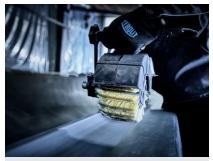
Tyrolit Power revolutionised the finishing of hard surfaces. Sanding strips consisting of layers made from cactus hair and diamond provide extreme hardness, save time and significantly reduce vibrations for the user.
